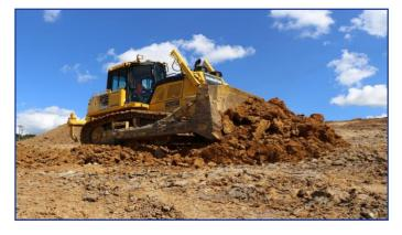
**Komatsu D65PXi-18 Fully Integrated Machine Control** Pat Blade, Idle Timer, Battery Isolator, Starter Isolator, Jump Start Connector Plug, Hi Visibility Labelling,9kg fire extinguisher,1 kg fire extinguisher in cab,ReversingCamera, Rippers,760mm grouser plates.
