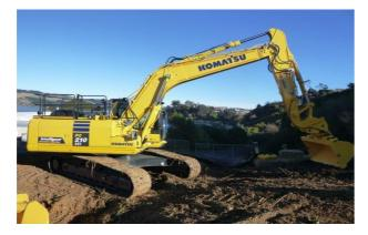
**Komatsu PC210LCi-10 Fully Integrated Machine Control** Fitted with Dig and Weed Buckets, Tilt and Breaker lines, Quick Hitch, Anti Drop Valves, 3 x Emergency Stop Switches, Hand Rails, Side Bump Rails, Hi Visibility Labelling, Battery Isolator, Starter Isolator, Jump Start Connection, Fire Extinguishers, Flashing Light, Full Length Sill Protection, ROP'S Cert Cab, FOP's Protection, Komtrax Tracking System.
