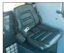
Trainer's seat diagonally behind the operator
