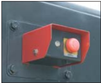
Emergency stop switch (with engine start lock function)
