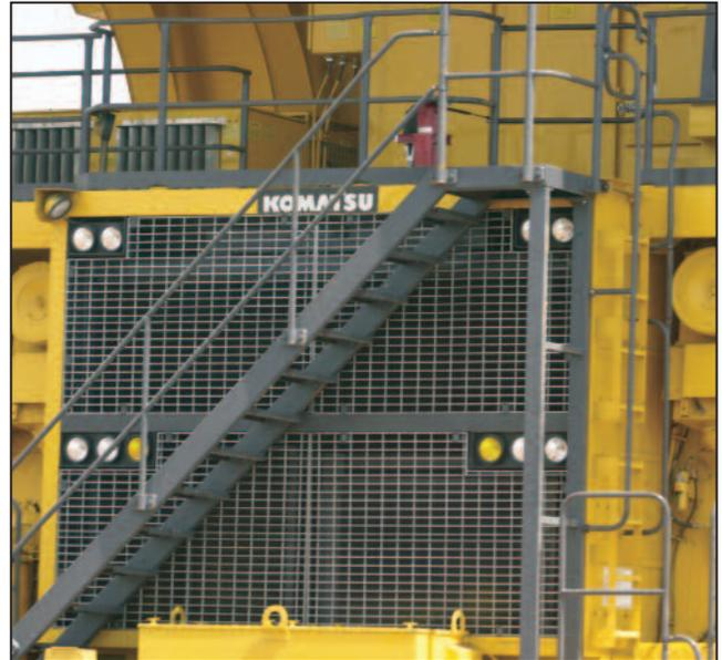
Komatsu's 960E-2 offers stairway access with entry from either the right or left side of the truck depending on the customer's preference.
