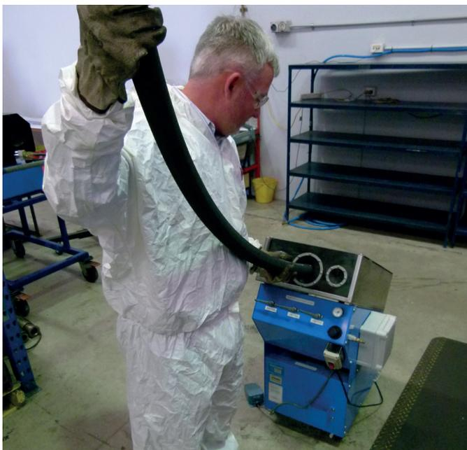
Specialised cleaning techniques to ensure the hose assembly is contaminant-free and all assemblies are individually bagged and capped to prevent damage and contamination of the assembly. All assemblies are clearly tagged to make re-ordering your hose simple and easy. Komatsu Engineering Standard (KES) assembly techniques ensures traceability of products and components that are used in the assembly process.
