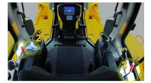
Note: Depending on the model and operator preference, the forward and reverse shift may be located next to the steering wheel 2a, next to the work equipment levers **2b**, or on models with joystick steering it will be on the steering lever.
