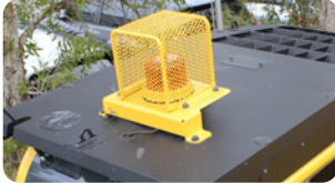
Rotating amber beacon Fitted with factory guard.
