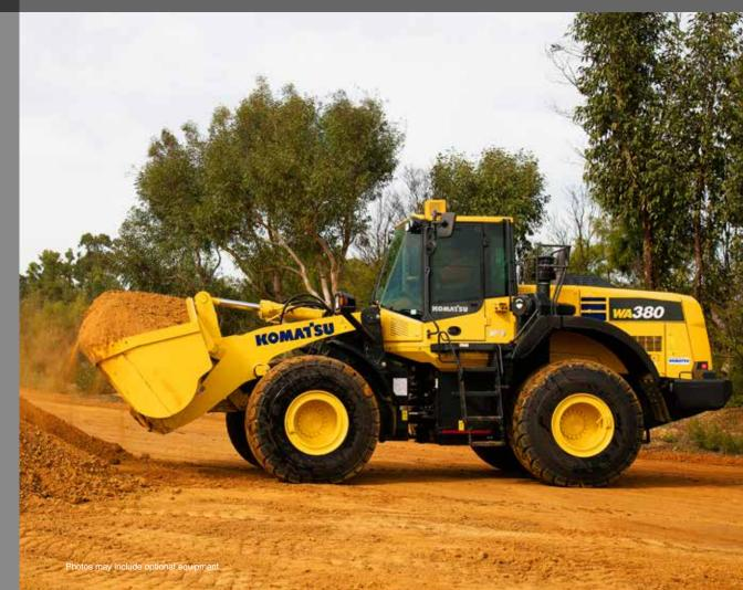
NET HORSEPOWER 143 kW / 191 HP @ 2100 rpm **OPERATING WEIGHT** 18,385 – 19,020 kg **BUCKET CAPACITY** 2.7 – 3.6 m<sup>3</sup>
