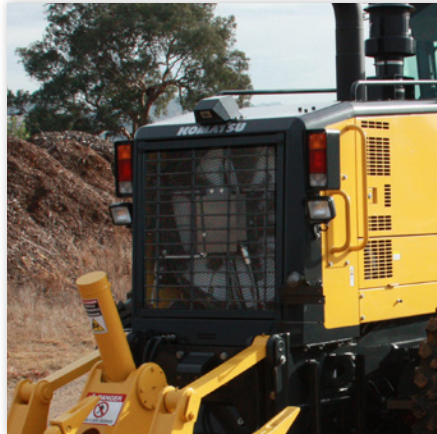
Easy radiator cleaning with reverse fan
