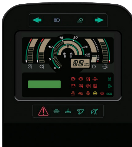
Console with central warning lamp. Internal monitoring system with error codes appearing in the display screen.
