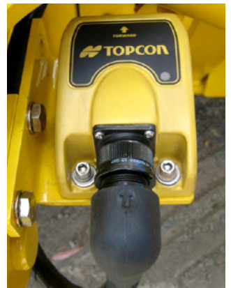
Topcon Cross Slope Sensor
