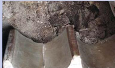
**Sprocket Teeth:** Minimal wear visible
