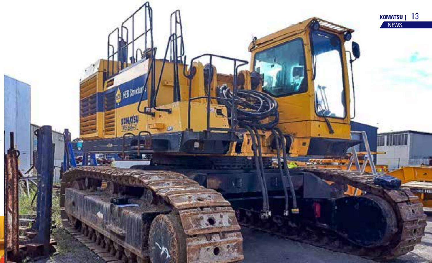
*Pictured: This PC1250, which suffered from the effects of working in close proximity to salt water, is having a major rebuild done.*
