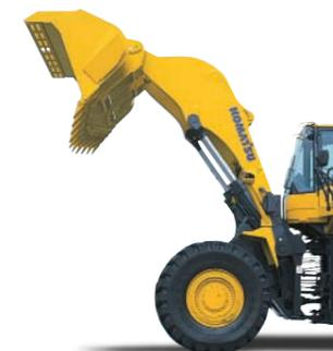
The WA600 can load 60t (70 Short ton) trucks with standard boom. The WA600-3 required an optional high lift boom and 6.4m<sup>3</sup> bucket. The WA600-6 maintains good visibility for loading because of increased operator cab height.
