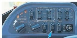
Dual mode engine power selection switch
