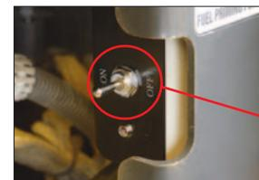
Electric priming pump switch
