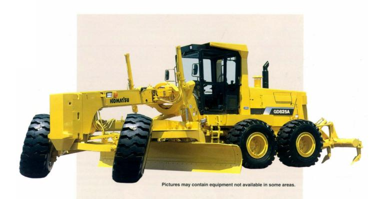
Flywheel Horsepower 209 kW (280 HP) Blade Length 4878 mm (16') Operating Weight 26350 kg (58,090 lb)
