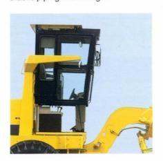
Note: Before using elevating mechanism, ask Komatsu distributor for instructions on the safe and proper way to lift cab.
