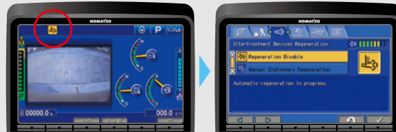
Aftertreatment device regeneration screen
