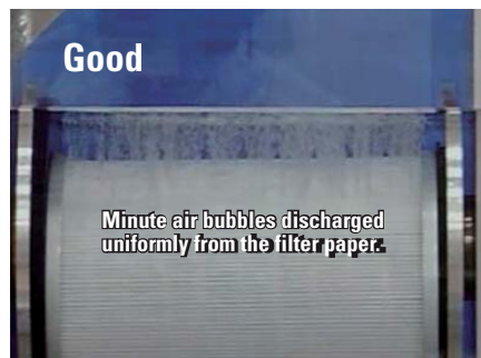
Minute air bubbles released from the surface of the filter paper.
